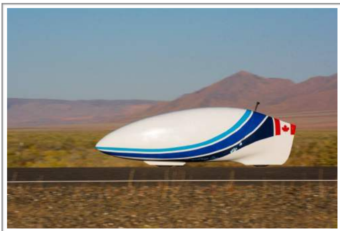
Eta Prime speedbike exceeding 100 km/h during a race at the World Speed Challenge
