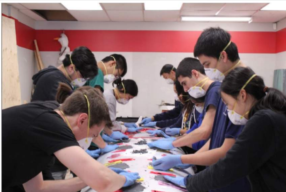
Concrete Canoe team members placing concrete onto the canoe mould during casting day.
