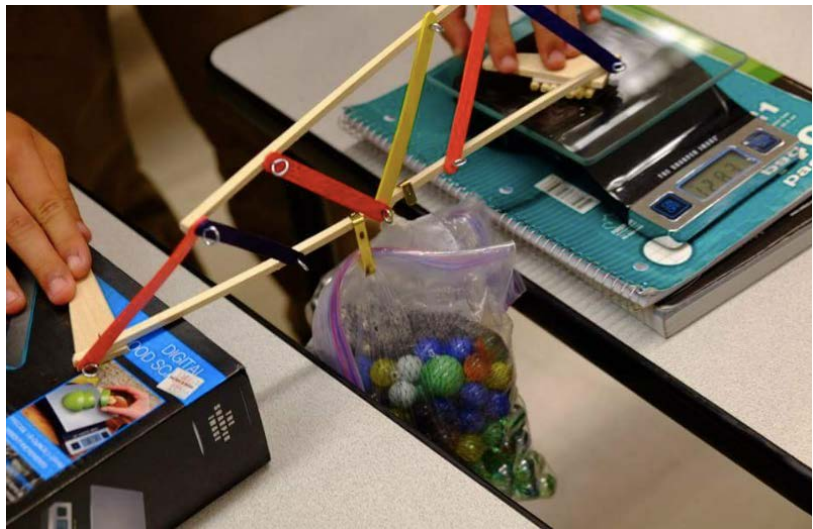
Truss Event: Loading a truss to failure
